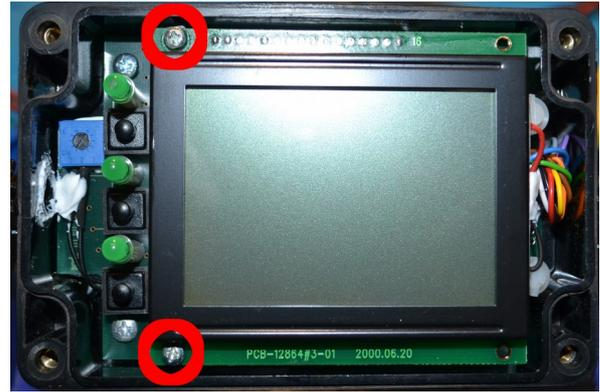
**Step 2:** Unplug the display by lifting it from the left side (where you just removed the two bolts).
