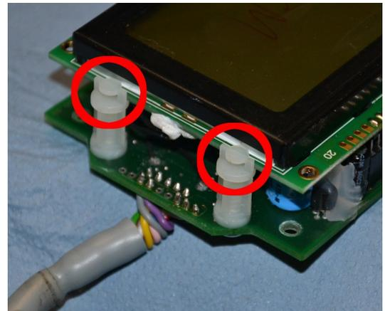
**Step 2:** Plug it back in, starting on the right hand side (when looking at the Tripmaster in normal viewing orientation) making sure that the pinheader and the connector are lined up properly. It is fairly easy to be off by one pin, therefore it is important to pay attention to this.
