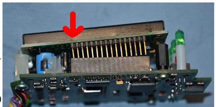
**Step 3:** Fully put the pinheader in the connector now, you'll feel a positive click when it is fully inserted.
